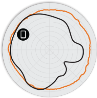
Figure 2. R320 2.4GHz Azimuth Antenna Patterns
